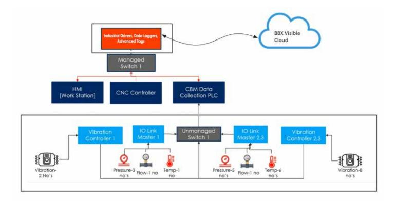
alerts and notifications. At the IoT platform, the data is now stored, processed, and continuously analyzed to trigger alerts or notifications. Reports can be generated in real-time and the BBX VISIBLE dashboard provides complete visualization of real-time data of all connected sensors and PLCs.
