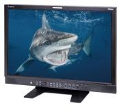
Developed from its HLM-2460W predecessor, the HLM-2460WA has a 1920x1200 pixel IPS LCD with 1,800:1 contrast ratio and 400 nits peak brightness. Features include PIP and side-by-side display, onscreen markers plus R/G/Y tally. UMD facilities are provided in addition to closed caption and VITC display. Test signals include waveform and vectorscope, dot-by-dot plus 2x/4x zoom. Audio capabilities include SDI audio de-embedding, eight-channel level metering and 5.1 down-mix.
