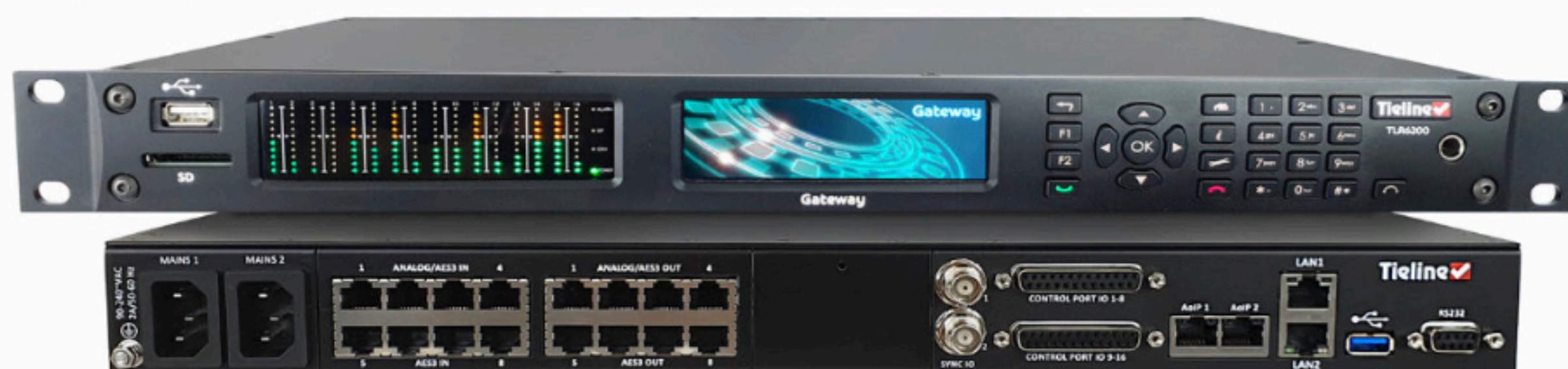
Tieline codecs such as the Gateway operate on the edge of IP networks, interfacing between studios and WANs like the internet
